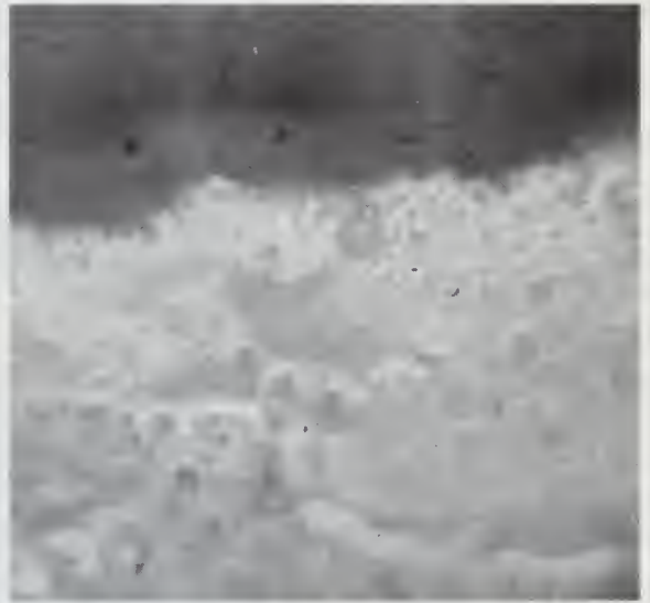
FIGURE 26. BIAxIAL COMPRESSIVE SPECIMEN FRACTURE SURFACE AT CRACK EDGE, CTBN R-151 (LARGE PARTICLES). (450X).
